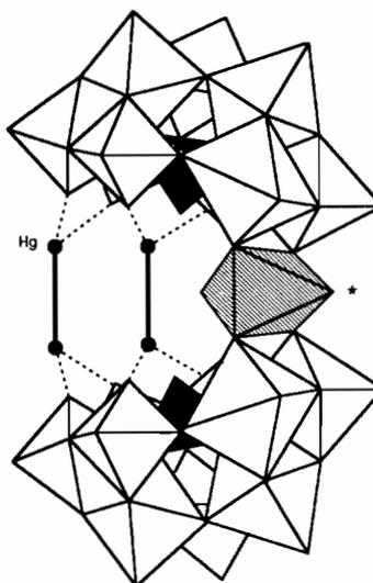
Fig. 8.  $[\text{As}^{\text{III}}_2(\text{Hg}^{\text{I}}_2)_2\text{W}_{19}\text{O}_{67}(\text{H}_2\text{O})]^{10-}$  polyanion.  $\text{AsO}_3$  groups are darkened. The octahedron joining the two  $\text{AsW}_9\text{O}_{33}$  moieties is dashed. The linkage of both  $(\text{Hg}^{\text{I}}_2)^{2+}$  cations to oxygen vertices is represented by dashed lines. The location of the water molecule is shown by an asterisk.
