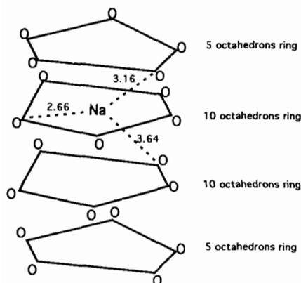
Fig. 20. Location of the oxygen atoms of the four tungsten rings which are inside the polyanion. It shows the sodium location and the 15 oxygen atoms surrounding sodium with Na–O distances.
