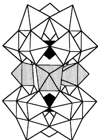
Fig. 6.  $[\text{As}^{\text{III}}_2\text{W}_{21}\text{O}_{69}(\text{H}_2\text{O})]^{6-}$  polytungstate. Two square pyramids and one octahedron keep separate the two  $\text{As}^{\text{III}}\text{W}_9\text{O}_{33}$  moieties, providing space for arsenic(III) lone pairs.  $\text{AsO}_3$  groups are darkened.
