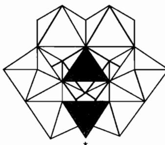
Fig. 12.  $[\text{As}^{\text{III}}_2\text{W}_8\text{O}_{30}(\text{OH})]^{7-}$  polyanion.  $\text{AsO}_3$  groups are darkened. Both lone pairs of arsenic(III) expand in the same direction, perpendicularly to the figure plane. The OH group is located at the free vertex of the  $\text{AsO}_3$  group which is at the bottom of the figure and marked by an asterisk.
