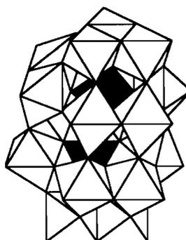
Fig. 3.  $[\text{P}_2\text{W}_{18}\text{O}_{62}]^{6-}$  polytungstate called Dawson structure.  $\text{PO}_4$  tetrahedrons are darkened.
