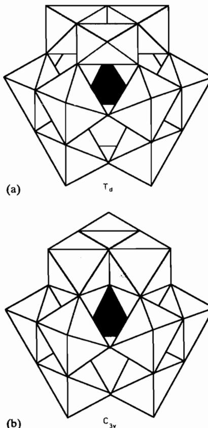
Fig. 1. Drawings of both  $\alpha$ - and  $\beta$ -isomers  $[\text{XW}_{12}\text{O}_{40}]^{n-}$ : (a) the Keggin structure of  $T_d$  symmetry; (b) the Sasaki structure of  $C_{3v}$  symmetry. The central  $\text{XO}_4$  tetrahedron is darkened. There is a turn of  $60^\circ$  of the shadowed  $\text{W}_3\text{O}_{13}$  group between both isomers.
