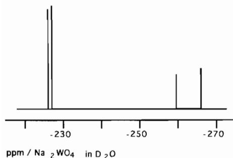
Fig. 19. Sketched NMR spectrum of  $[\text{NaP}_5\text{W}_{30}\text{O}_{110}]^{14-}$ . Because sodium is at the centre of a ten tungsten atoms ring, those two ten tungsten rings are not NMR equivalent, as well as those of the two five tungsten rings. Consequently there are four peaks with 1–1–2–2 heights. The  $^{183}\text{W}$  resonance frequency was 16.67 MHz.
