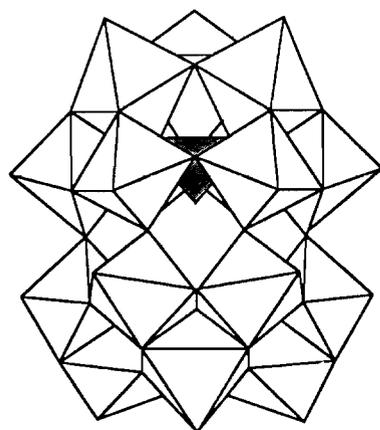
Fig. 5.  $[\text{As}^{\text{III}}\text{H}_2\text{W}_{18}\text{O}_{60}]^{7-}$  polytungstate; the arsenic(III) is bound to three oxygens only. The  $\text{AsO}_3$  group is darkened. The lone pair expands in the  $\text{W}_9\text{O}_{33}$  moiety which does not contain any arsenic.
