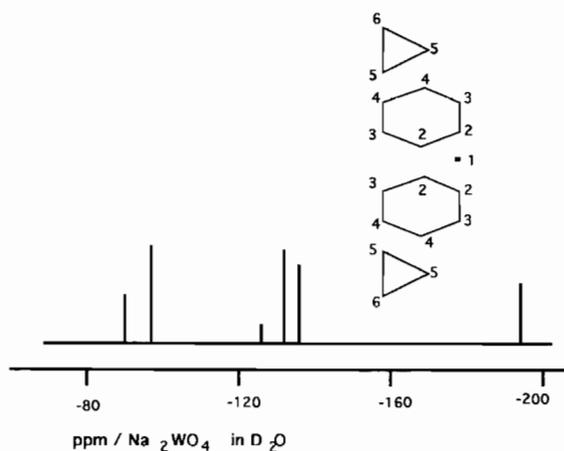
Fig. 10. Sketched NMR spectrum of  $[\text{As}^{\text{III}}_2(\text{Hg}^{\text{I}}_2)_2\text{W}_{19}\text{O}_{67}(\text{H}_2\text{O})]^{10-}$ . The diagram presents the six different types of tungsten atoms marked as 1, 2, 3, 4, 5, 6, numbering 1 the octahedrally surrounded tungsten atom joining the two  $\text{AsW}_9\text{O}_{33}$  moieties. The  $^{183}\text{W}$  resonance frequency was 16.67 MHz.
