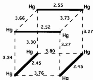
Fig. 9. The asymmetric unit contains two polyanions  $[\text{As}^{\text{III}}_2(\text{Hg}^{\text{I}}_2)_2\text{W}_{19}\text{O}_{67}(\text{H}_2\text{O})]^{10-}$  at  $90^\circ$ . The eight mercury atoms are at vertices of a distorted cube; intra and inter polyanionic  $\text{Hg}\cdots\text{Hg}$  non-bonding distances are nearly identical.
