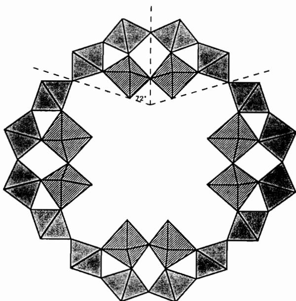
Fig. 17. Projection of the  $[\text{P}_8\text{W}_{48}\text{O}_{184}]^{40-}$  polyanion. Octahedrons are not transparent; one half of them is seen, each octahedron hiding another one located underneath. Phosphorus atoms are represented by black dots.  $\text{PW}_6\text{O}_{26}$  group is limited by two planes which make a dihedral angle of  $72^\circ$ . Four  $\text{P}_2\text{W}_{12}\text{O}_{48}$  groups make a large ring.
