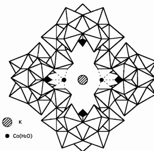
Fig. 11.  $[\text{As}^{\text{III}}_4\text{Co}_2\text{KW}_{40}\text{O}_{140}]^{28-}$  polyanion. The four  $\text{AsO}_3$  groups are darkened. Cobalt atoms are shown by large black dots. The potassium atom is at the centre of the polyanion and shown by a dashed circle. The four  $\text{WO}_6$  octahedrons joining the four  $\text{AsW}_9\text{O}_{33}$  moieties and providing the flexibility to the whole structure, are shadowed.
