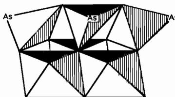
Fig. 13.  $[As^{III}_3Mo_3O_{15}]^{3-}$  polyanion. The three arsenic(III) form a chained anion  $O_2AsOAs(O)OAsO_2^{5-}$  anion stretching above the  $Mo_3O_{13}$  group and sharing with it five oxygen atoms.
