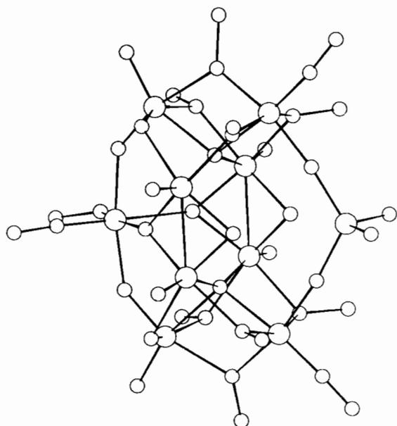
Fig. 27. Molecular structure of the anion  $[\text{Mo}_{10}\text{O}_{20}(\text{OMe})_9(\text{NO})_3]^{2-}$ . It contains one  $\text{MoO}_4$  group. There are four  $\text{Mo}^{\text{V}}$  bonded two by two with a 2.57 Å Mo–Mo distance. There are three  $\text{Mo}^{\text{II}}(\text{NO})$  groups. One of them is in a  $\text{Mo}(\text{NO})\text{O}_4(\text{OMe})$  octahedron, two oxygens of which each bridge a  $\text{Mo}^{\text{V}}\text{--}\text{Mo}^{\text{V}}$  bonded pair.
